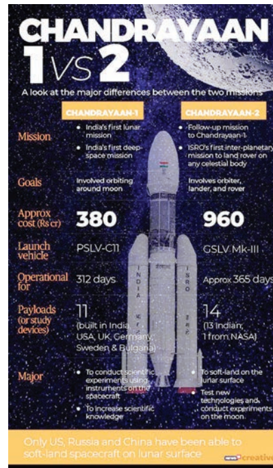
A look at major differences between Chandrayaan-1 which was launched by ISRO in October 2008 and Chandrayaan 2 launched on 22 July 2019
