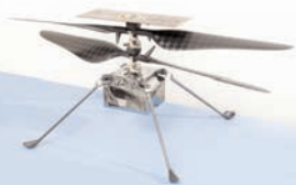
The flight model of NASA's Ingenuity Mars Helicopter - Image: NASA / JPL
