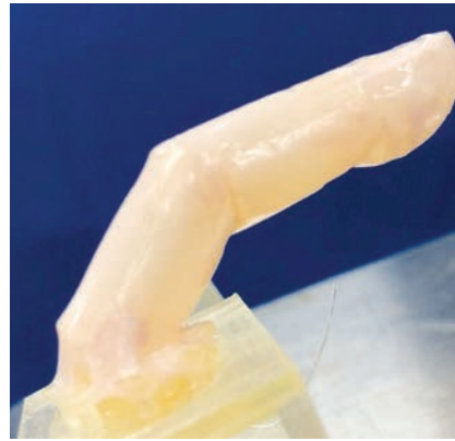
The articulated robot finger covered with living skin tissue that can self-heal with the help of a collagen bandage is seen in Tokyo, Japan, in this undated handout photo released by Biohybrid Systems(Takeuchi) Laboratory, The University of Tokyo and obtained by Reuters on June 10, 2022. Biohybrid Systems(Takeuchi) Laboratory, The University of Tokyo/Handout via Reuters
