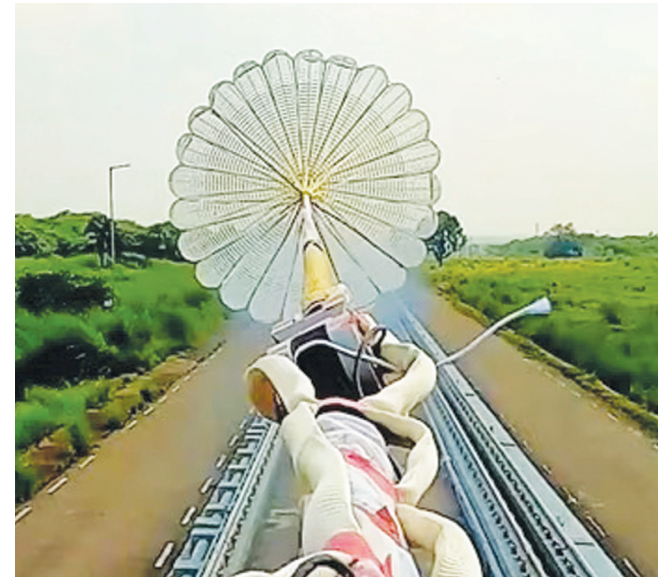
ISRO conducts tests on drogue parachutes (ISRO)
